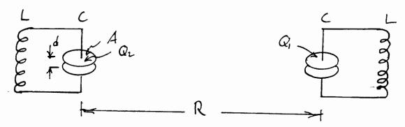
$$L\ddot{Q}_1 + \frac{Q_1}{C} = \frac{Q_2 d^2}{R^3}; \qquad L\ddot{Q}_2 + \frac{Q_2}{C} = \frac{Q_1 d^2}{R^3}.$$
