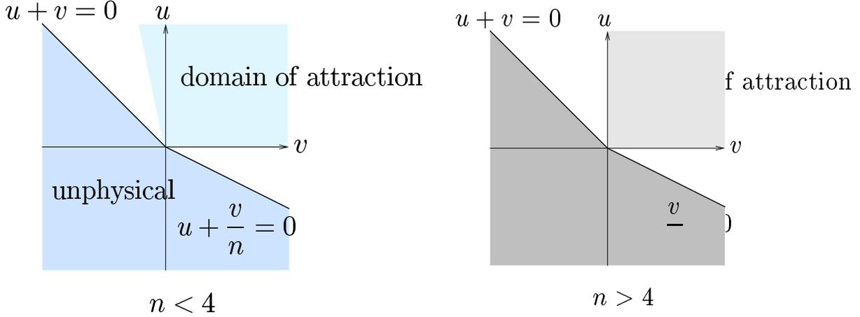
Flows which are not originally located within these domains of attraction flow into the unphysical regions. The coupling constants  $u$  and  $v$  become more negative. This is the signal of a fluctuation induced first order phase transition, by what is known as the Coleman–Weinberg mechanism. Fluctuations are responsible for the change of order of the transition in the regions of the  $(u, v)$  plane outside the domain of attraction of the stable fixed points.
