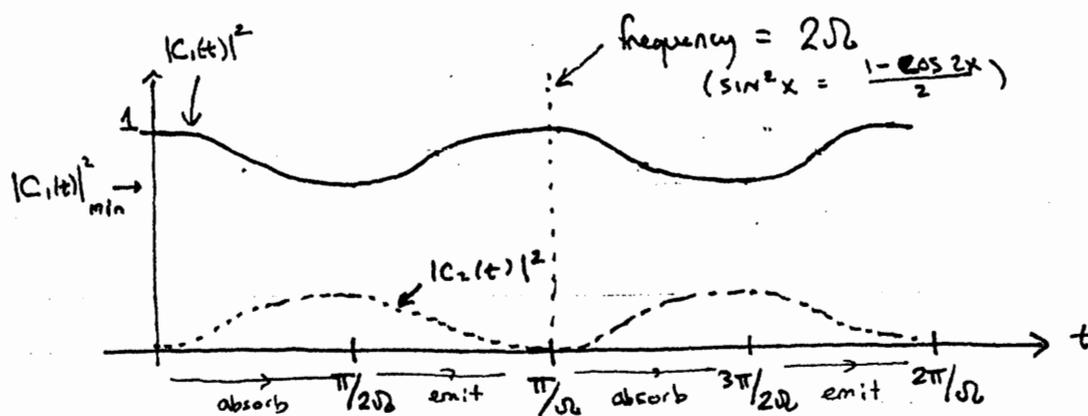
$$|C_1(t)|^2_{\min} = \frac{(\omega - \omega_{z1})^2}{(\omega - \omega_{z1})^2 + 4\Gamma^2/\kappa^2}$$
