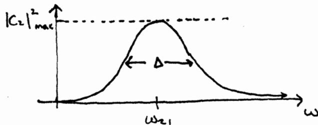
$$\begin{aligned} \Delta &= \text{full width @ half max} \\ &= 4\Gamma/\kappa \end{aligned}$$
