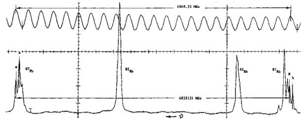
FIG. 7: Panoramic spectrum and interferogram for determination of  $5^2S_{1/2}$  hfs. Please note that this particular spectrum was obtained using a research grade instrument and your own spectra may not look quite as nice.
