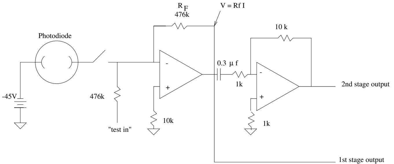
FIG. 7: Diagram of the photo-diode and preamplifier circuit.
