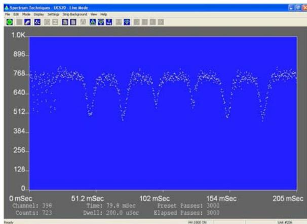
FIG. 7: Typical Mossbauer spectrum using an enriched Fe-57 foil acquired by the Spectech UCS-20 multi-channel analyzer. Distance between Co-57 and proportional counter detector window is  $\sim 10$ cm. Integration time = 3000 passes  $\sim 10$  minutes. Co-57 had  $\sim 5$ mCi of activity.
