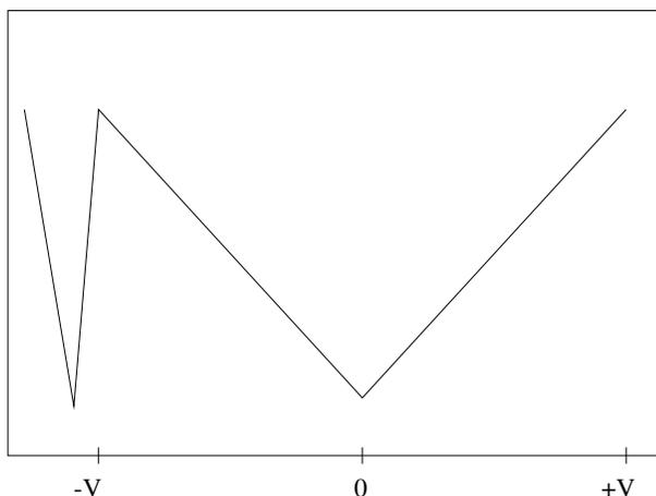
FIG. 9: Ideal appearance of the multichannel scaler screen after several minutes of operation with the interferometer velocity calibrator. The sharp feature at the start is produced during the rapid reversal of the velocity of the piston at the high speed end of its stroke. In reality, the bottom of the “V” will probably be truncated due to the low amplitude of the pulses during the low-velocity portion of the sweep.
