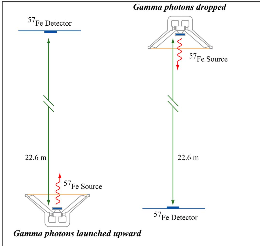
Over 22.6 meters, the **gravitational redshift** is only  $5 \times 10^{-15}$ , but the **Mössbauer effect** with the 14.4 keV  $\gamma$ -ray from **iron-57** has a high enough resolution to detect that difference.
