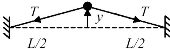
The vertical component of the tension in both strings is driving the mass back to equilibrium (see figure).
