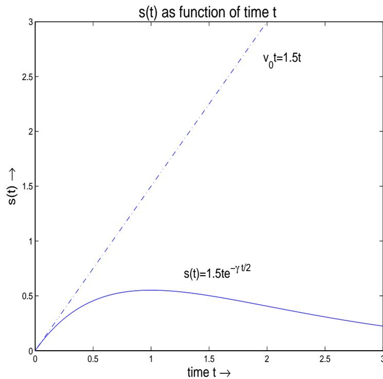
FIG. 4: 1.9(a) Plot of  $s(t)$  in the critically damped system
