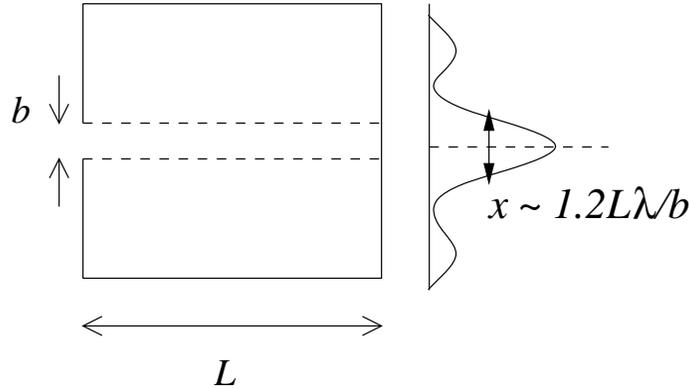
A distant source produces a Fraunhofer diffraction pattern on the screen with a central maximum width
