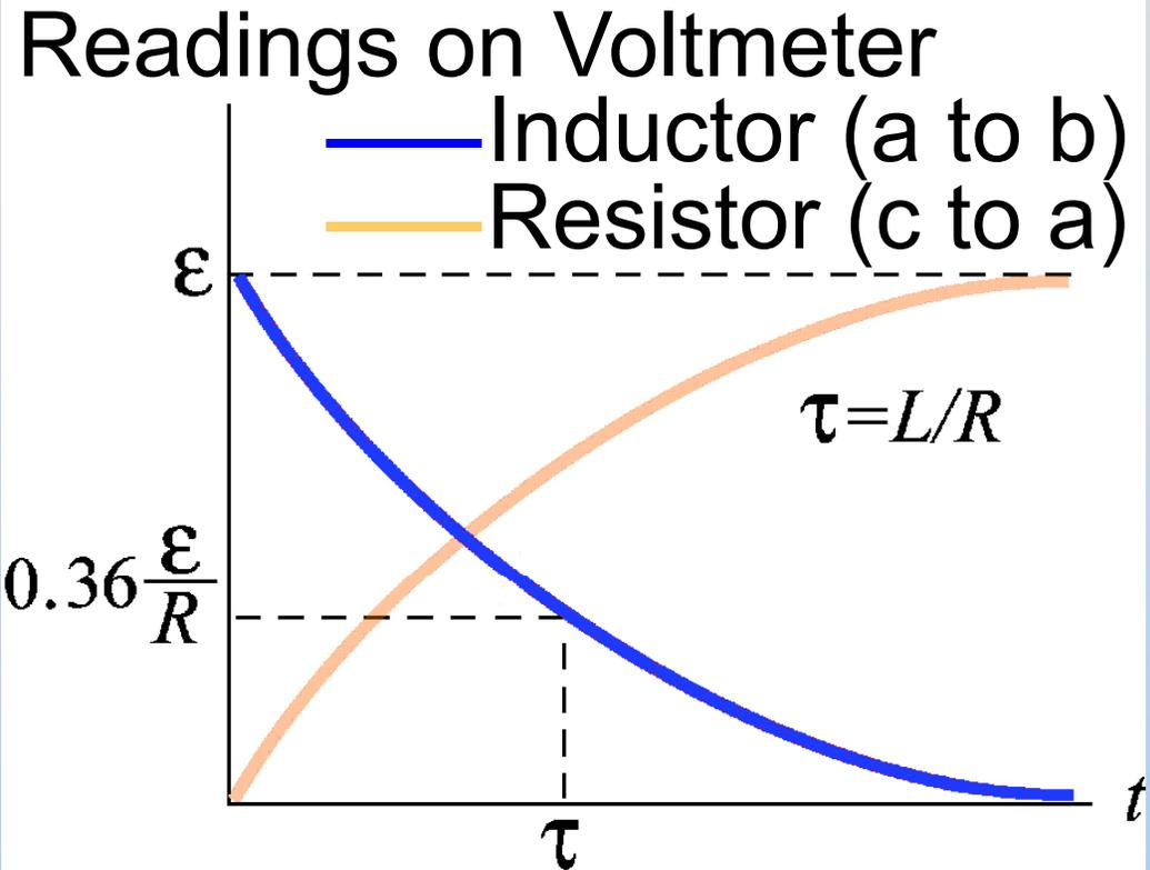
$t=0^+$ : Current is trying to change. Inductor works as hard as it needs to to stop it
