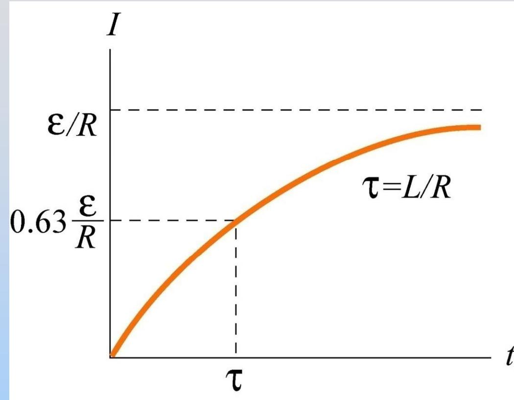
$t=0^+$ : Current is trying to change. Inductor works as hard as it needs to to stop it
