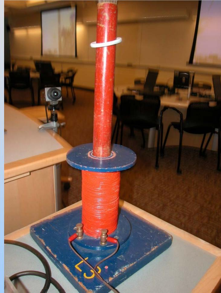
It looks as though the conducting loops have current in them (they behave like magnetic dipoles) even though they aren't hooked up
