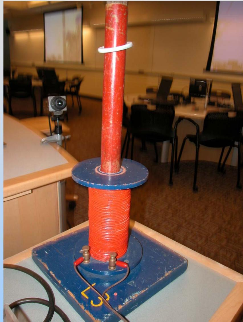
An aluminum ring jumps into the air when the solenoid beneath it is energized
