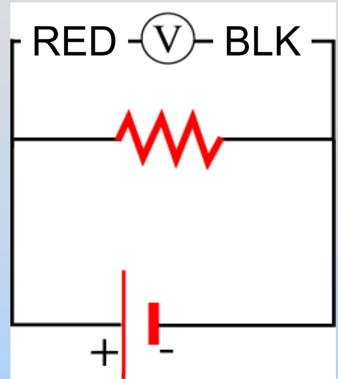
1. Hook in PARALLEL: reads  $V_{\text{Red}} - V_{\text{Black}}$
