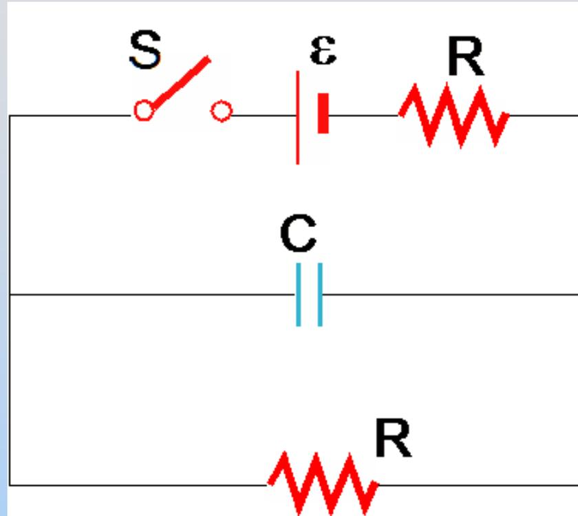
For the above circuit sketch the currents through the two bottom branches as a function of time (switch closes at  $t = 0$ , opens at  $t = T$ ). State values at  $t = 0^+$ ,  $T^-$ ,  $T^+$
