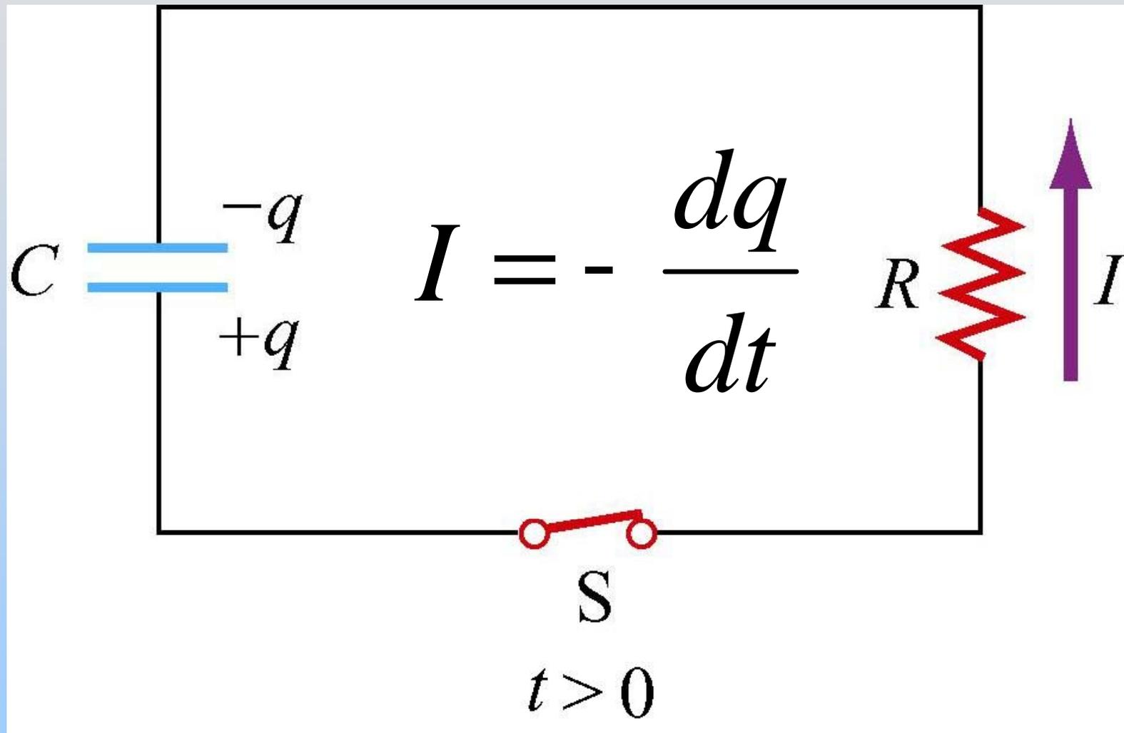
$$\sum_i \Delta V_i = \frac{q}{C} - IR = 0 \quad \sum_i \Delta V_i = \frac{q}{C} + \frac{dq}{dt} R = 0$$
