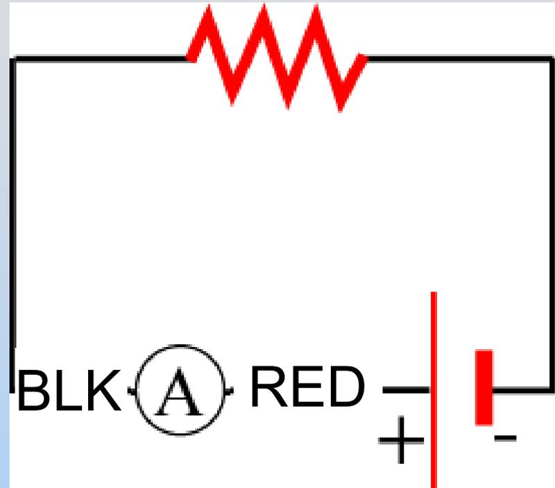
1. Hook in **SERIES**: current must go thru to measure
