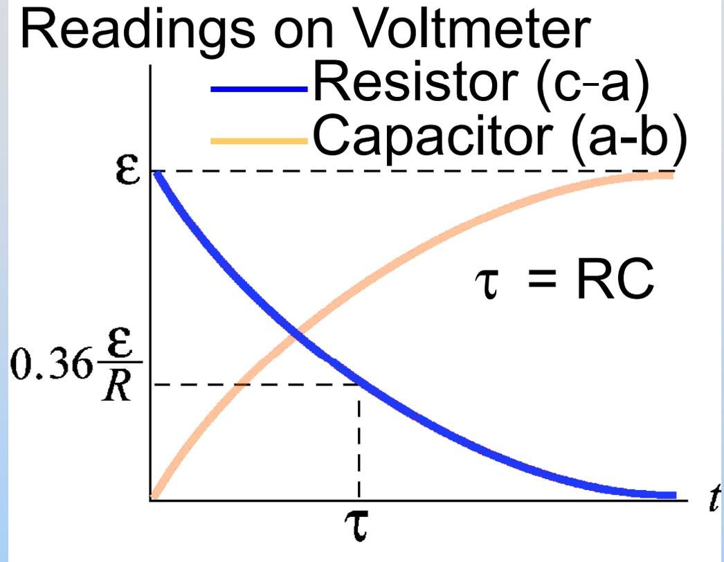
$t=0^+$ : Capacitor is uncharged so resistor sees full battery potential and current is largest
