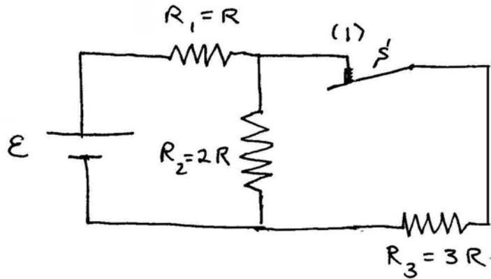
Resistors 2 and 3 are now in parallel with equivalent resistance
