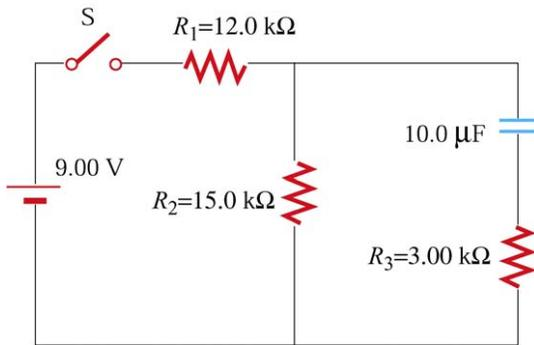
(a) Find the steady-state current in each resistor.
