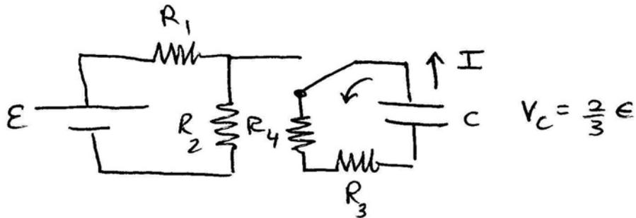
The current flows counterclockwise (up from the capacitor). Because  $|V_C| = (2/3)\varepsilon$  and the equivalent resistance is  $R_{eq} = R_4 + R_3 = 4R$ , the current is
