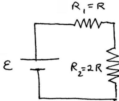
In this single loop circuit with equivalent resistance  $R_{eq} = R_1 + R_2 = 3R$ , the current is the same through both resistors with resistances  $R_1$ ,  $R_2$ , and is given by  $I = \mathcal{E}/(3R)$ .
