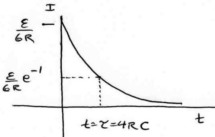
(e) Because the equivalence resistance is  $R_{eq} = 4R$ , the time constant is
