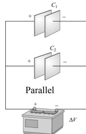
uncharged when the capacitors are connected (which is always the case unless otherwise stated). In parallel, the capacitors have the same potential drop across them (their bottoms and tops are at the same potential). From these setups we will calculate the equivalent capacitance of the system – what one capacitor could replace the two capacitors and store the same amount of charge when hooked to the same battery. It turns
