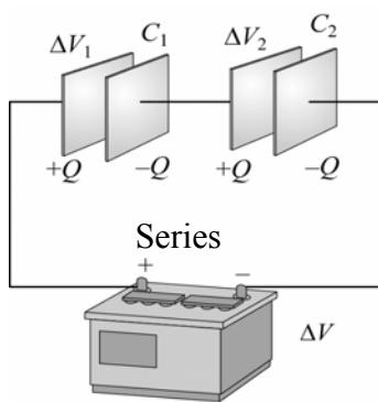
Last time we introduced the idea of a capacitor as a device to store charge. This time we will discuss what happens when multiple capacitors are put together. There are two distinct ways of putting circuit elements (such as capacitors) together: in *series* and in *parallel*. Elements in series (such as the capacitors and battery at left) are connected one after another. As shown, the charge on each capacitor must be the same, as long as everything is initially
