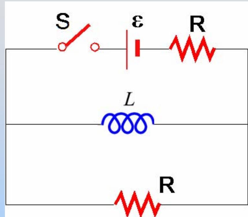
For the two above circuits sketch the currents through the two bottom branches as a function of time (switch closes at  $t = 0$ , opens at  $t = T$ ). State values at  $t = 0^+$ ,  $T^-$ ,  $T^+$
