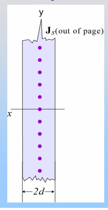
A sheet of current (infinite in the y & z directions, of thickness 2d in the x direction) carries a uniform current density:
