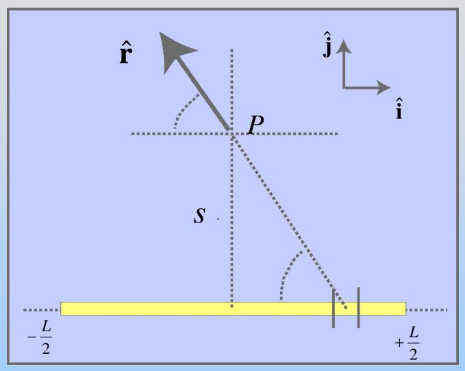
Point *P* lies on perpendicular bisector of uniformly charged line of length *L*, a distance *s* away. The charge on the line is *Q*. What is *E* at *P*?
