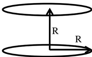
As pictured at left, a Helmholtz coil is created by placing two such coils (each of radius  $R$  and  $N$  turns) a distance  $R$  apart.
