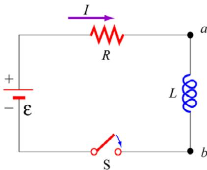
Consider the circuit at left, consisting of a battery (emf  $\epsilon$ ), an inductor  $L$ , resistor  $R$  and switch  $S$ .
