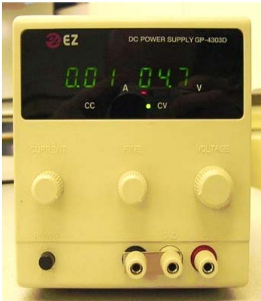
**Figure 4 Power Supply for Helmholtz Coil**
