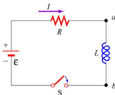
**Figure 5 RL circuit.** For  $t < 0$  the switch  $S$  is open and no current flows in the circuit. At  $t = 0$  the switch is closed and current  $I$  can begin to flow, as indicated by the arrow.
