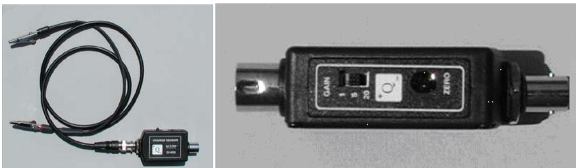
**Figure 5** Charge Sensor – measures voltage difference between its red and black leads. Left: Shown attached to the lead assembly. Right: The gain switch (used to amplify small signals) should be set at 1. The zero button sets the output signal to zero.
