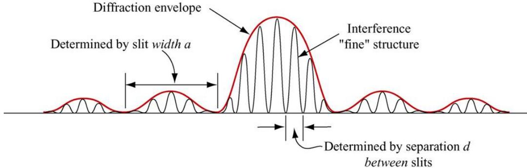
Here the amplitude modulation (the red envelope) is set by the diffraction (the width of the slits), while the “individual wiggles” are due to the interference between the light coming from the two different slits. You know that this must be the case because  $d$  must be larger than  $a$ , and hence the minima locations, which go like  $1/d$ , are closer together for the two slit pattern than for the single slit pattern.
