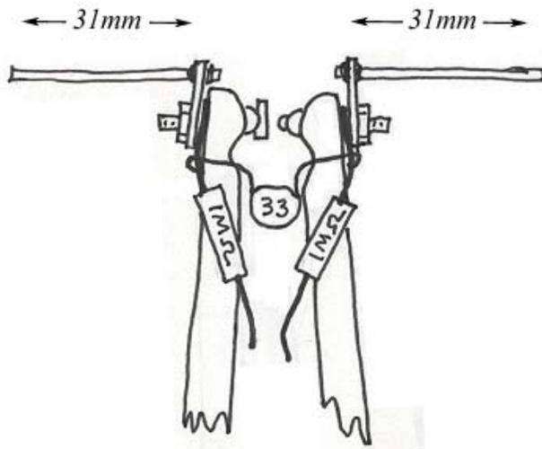
**Figure 1 Spark-gap transmitter.** The "33" is a 33 pF capacitor. It is responsible for storing energy to be rapidly discharged across a "spark gap," formed by two tungsten cylinders pictured directly above it (one with a vertical axis, one horizontal). Two M $\Omega$  resistors limit current off of the capacitor and back out the leads, protecting the user from shocks from the 800 V to which the capacitor will be charged. They also limit radiation at incorrect frequencies.
