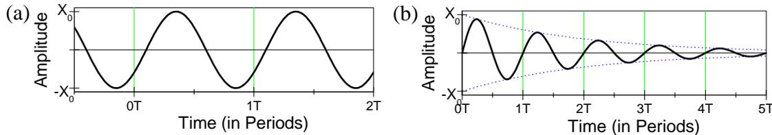
**Figure 1 Oscillating Functions.** (a) A purely oscillating function  $x = x_0 \sin(\omega t + \phi)$  has fixed amplitude  $x_0$ , angular frequency  $\omega$  (period  $T = 2\pi/\omega$  and frequency  $f = \omega/2\pi$ ), and phase  $\phi$  (in this case  $\phi = -0.2\pi$ ). (b) The amplitude of a damped oscillating function decays exponentially (amplitude *envelope* indicated by dotted lines)
