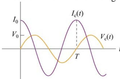
**Figure 4 Current and Voltage for a Capacitor**
