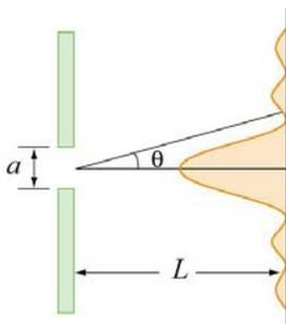
The next kind of interference we consider is light going through a single slit, interfering with itself. This is called diffraction, and arises from the finite width of the slit ( $a$  in the picture at left). The resultant effect is not nearly as easy to derive as that from two-slit interference (which, as you can see from above, is straight-forward). The result for the angular locations of the minima is  $a \sin(\theta) = m\lambda$ .
