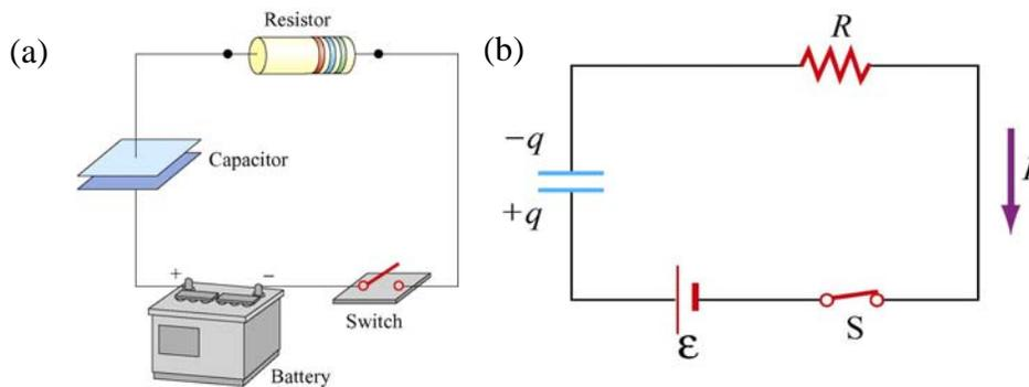
**Figure 2** (a) RC circuit (b) Circuit diagram for  $t > 0$
