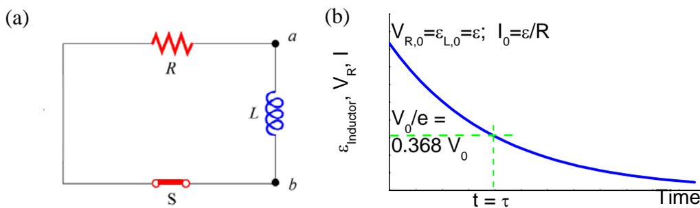
**Figure 7** Once (a) the battery is turned off, the EMF induced by the inductor and hence the voltage across the resistor and current in the circuit all (b) decay exponentially. The time constant  $\tau$  is how long it takes for a value to drop by  $e$ .
