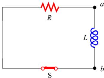
After a long time  $T$  the current will reach an equilibrium value and inductor will be “fully charged.” At this point we turn off the battery ( $\mathcal{E}=0$ ), allowing the inductor to ‘discharge,’ as pictured at left. Repeat each of the steps a-c in problem 4, noting that instead of  $\exp(-t/\tau)$ , our expression for current will now contain  $\exp(-(t-T)/\tau)$ .
