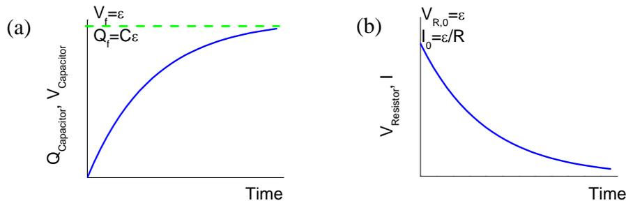
**Figure 3** (a) Voltage across and charge on the capacitor increase as a function of time while (b) the voltage across the resistor and hence current in the circuit decrease.
