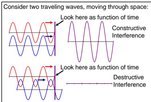
The picture at left forms the basis of all the phenomena you will observe in the lab. Two different waves arrive at a single position in space (at the screen). If they are in phase then they add constructively and you see a bright spot. If they are out of phase then they add destructively and you see nothing (dark spot).
