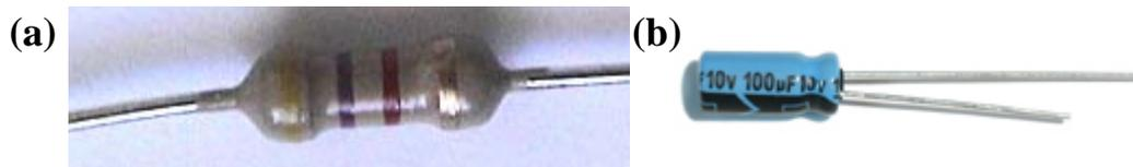
**Figure 10** Examples of a (a) resistor and (b) capacitor. Aside from their size, most resistors look the same, with 4 or 5 colored bands indicating the resistance. Capacitors on the other hand come in a wide variety of packages and are typically stamped both with their capacitance and with a maximum working voltage.
