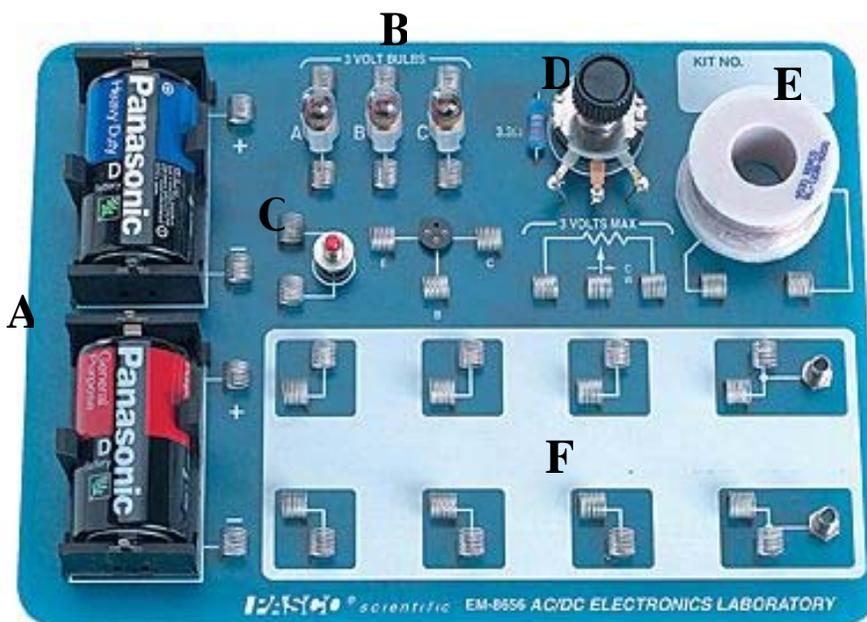
**Figure 8** The AC/DC Electronics Lab Circuit Board, with (A) Battery holders, (B) light bulbs, (C) push button switch, (D) potentiometer, (E) inductor and (F) connector pads
