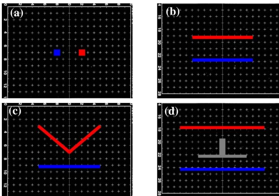
**Figure 2 Conducting Paper Landscapes.** Each of the four landscapes – the “standard” (a) dipole and (b) parallel plates, and the “non-standard” (c) bent plate and (d) filled plates – consists of two conductors which will be connected to the positive (red) and ground (blue) terminals of a battery. In (d) there is an additional conductor which is free to float to whatever potential is required. The pads are painted on conducting paper with a 1 cm grid.
