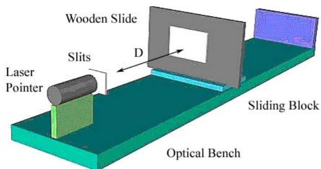
The optical bench consists of a holder for a laser pointer, a mount for slides (which contain the slits you will shine light through), and a sliding block to which you will attach pieces of paper to mark your observed interference patterns. Note that a small ring can be slid over the button of the laser pointer in order to keep it on while you make your measurements.
