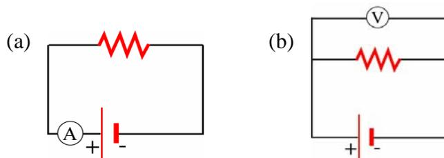
**Figure 1: Measuring current and voltage in a simple circuit.** To measure current *through* the resistor (a) the ammeter is placed in series with it. To measure the voltage drop *across* the resistor (b) the voltmeter is placed in parallel with it.
