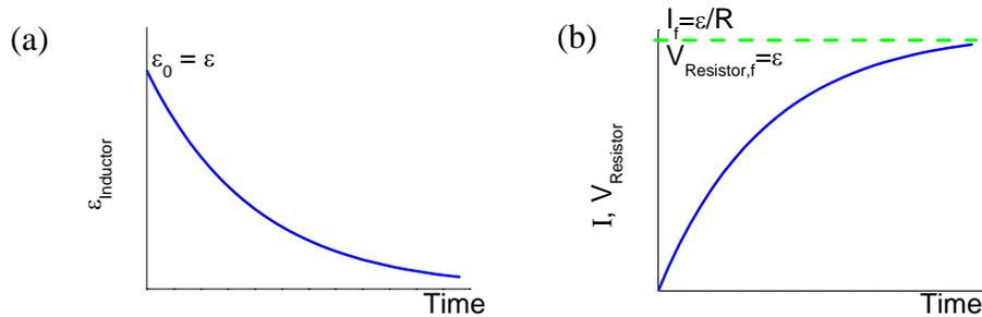
**Figure 6** (a) “EMF generated by the inductor” decreases with time (this is what a voltmeter hooked in parallel with the inductor would show) (b) the current and hence the voltage across the resistor increase with time, as the inductor ‘relaxes.’
