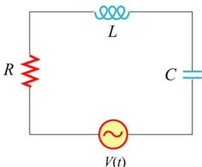
Consider the circuit at left, consisting of an AC function generator ( $V(t) = V_0 \sin(\omega t)$ , with  $V_0 = 5$  V), an inductor  $L = 8.5$  mH, resistor  $R = 5$   $\Omega$ , capacitor  $C = 47$   $\mu$ F and switch  $S$ .
