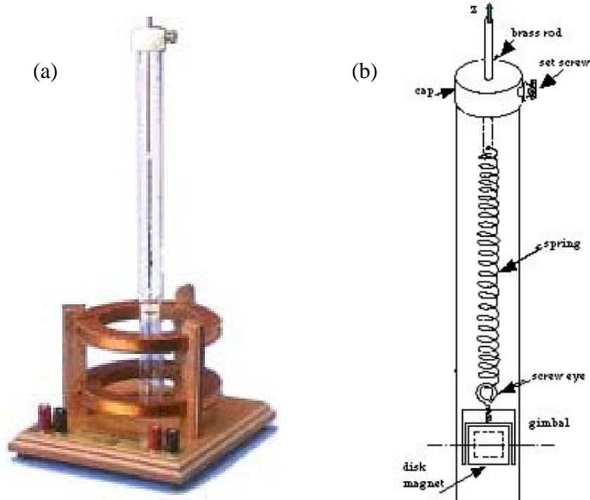
**Figure 1 The Teach Spin Apparatus** (a) The Helmholtz apparatus has a tower assembly (b) placed along its central axis. The tower contains a disk magnet which is free to rotate (on a gimbal) about an axis perpendicular to the tube and constrained to move vertically. The amount of motion can be converted into a force knowing the spring constant of the spring.
