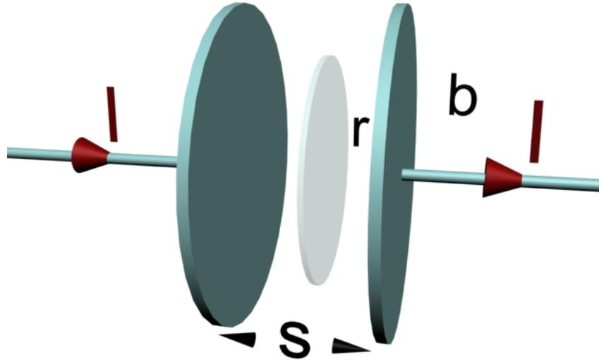
Consider the above circular capacitor, and the Amperian loop (radius  $r$ ) in the plane midway between the plates. When the capacitor is charging, the line integral of the magnetic field around the Amperian loop is
