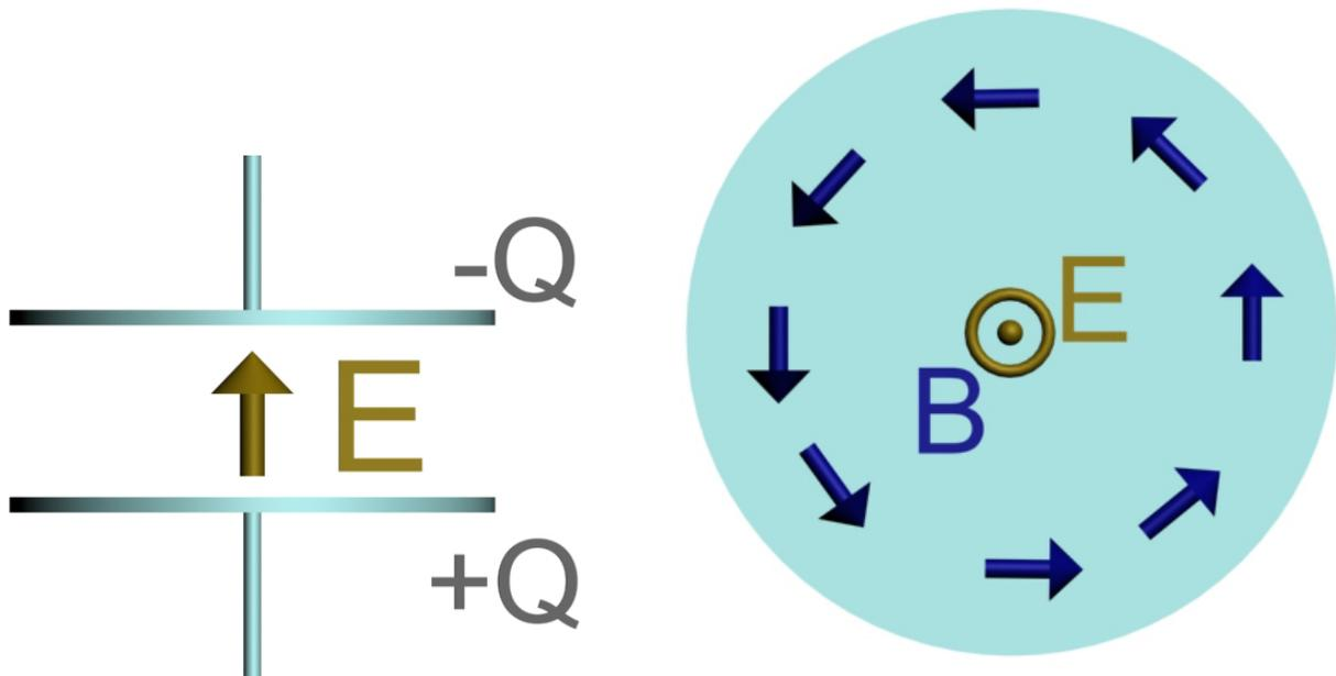
The plot above shows a side and a top view of a capacitor with charge  $Q$  with electric and magnetic fields  $E$  and  $B$  at time  $t$ . The charge  $Q$  is:
