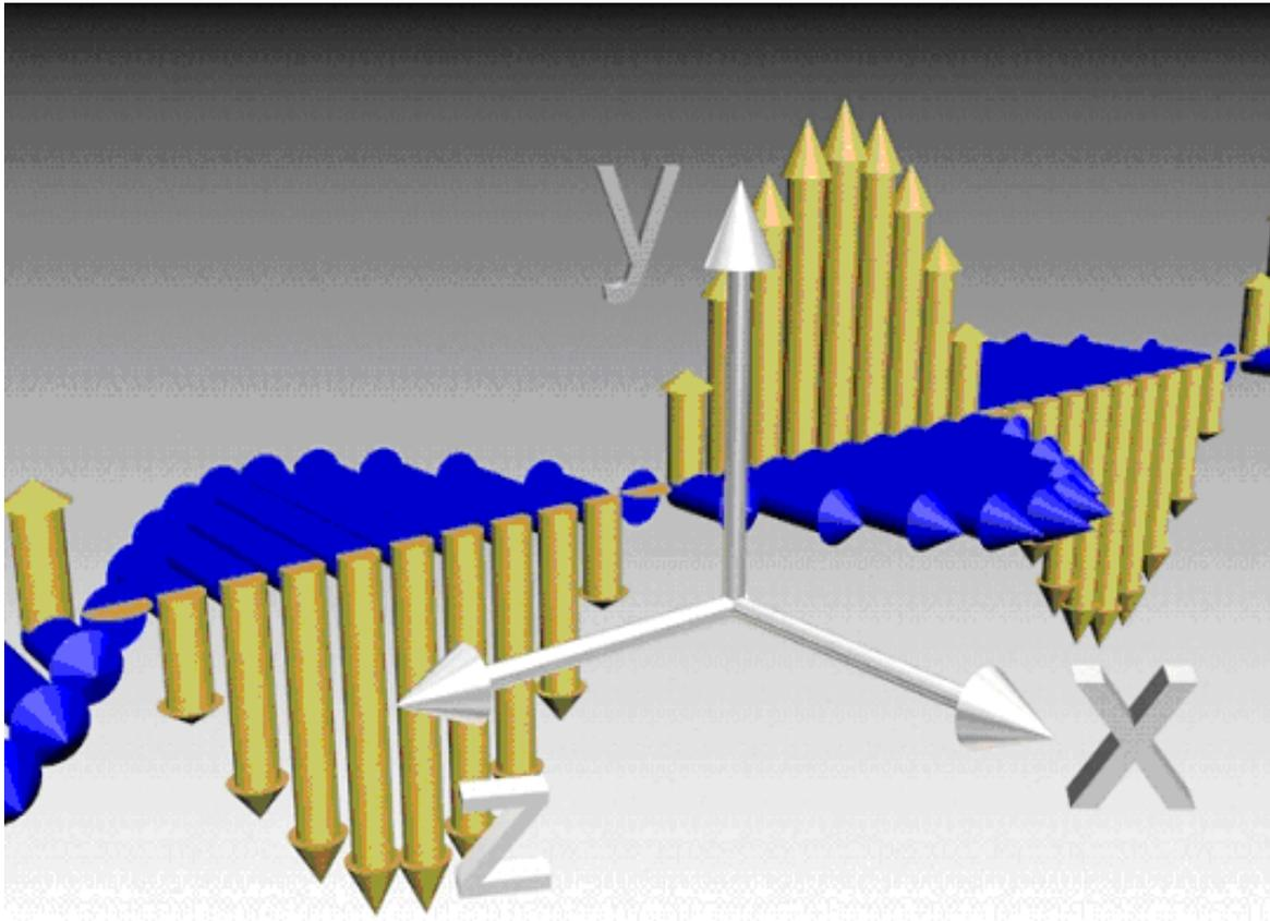
**The graph shows the E (yellow) and B (blue) fields of a plane wave. This wave is propagating in the**
