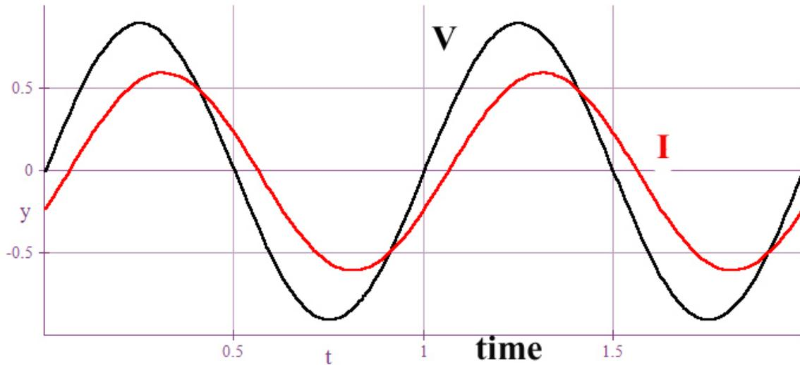
**The graph shows the current versus the voltage in a driven RLC circuit at a particular driving frequency. Is this frequency above or below the resonance frequency of the circuit?**
