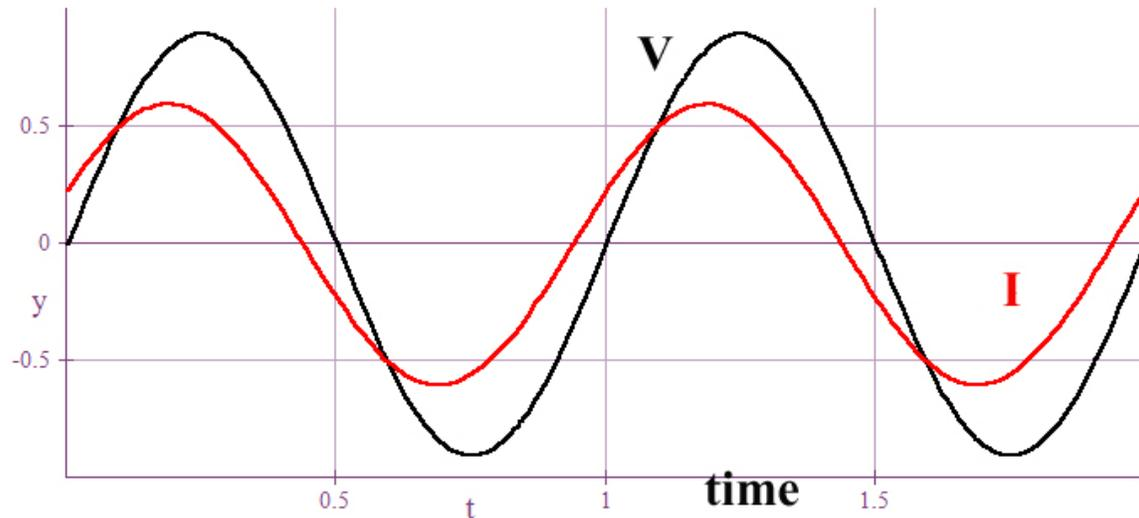
**The graph shows the current versus the voltage in a driven RLC circuit at a particular driving frequency. At this frequency, the circuit is dominated by its**
