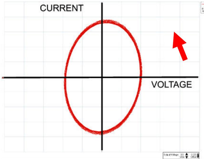
**The graph shows the current versus the voltage in a driven RLC circuit at a given driving frequency. In this plot**
