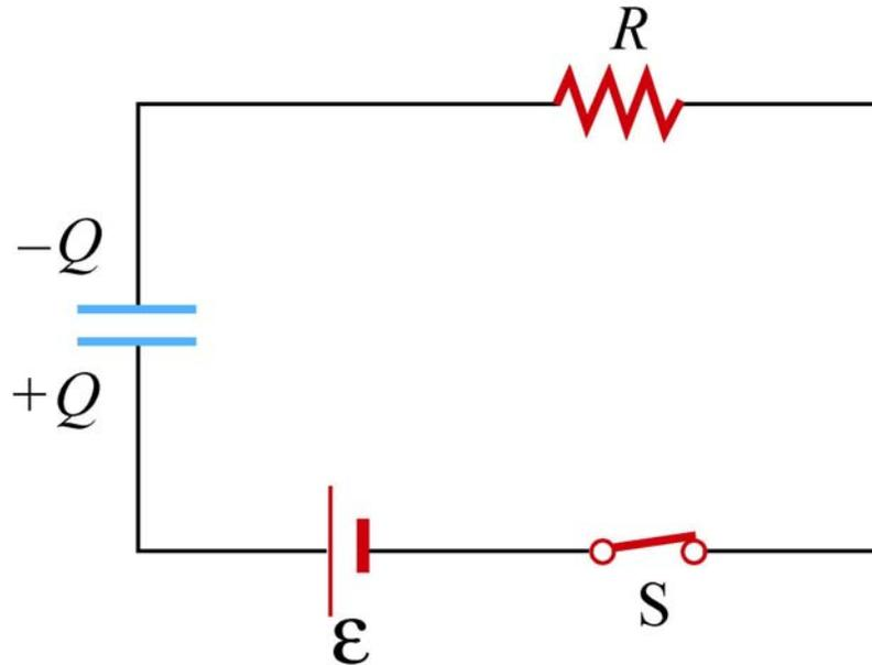
An uncharged capacitor is connected to a dc voltage source via a switch. A resistor is placed in series with the capacitor. The switch is initially open. At  $t = 0$ , the switch is closed. Just after the switch is closed, the current in the circuit is
