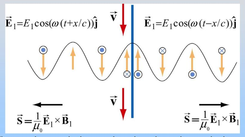
The work you do in moving the sheet is carried away as electromagnetic radiation, with 100% efficiency.
