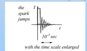
$$f_{\text{rad}} = \frac{1}{T} = \frac{c}{4l} = \frac{3 \times 10^{10} \text{ cm/s}}{12.4 \text{ cm}}$$
