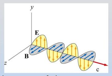
At every point in the wave and any instant of time, E and B are in phase with one another, with
