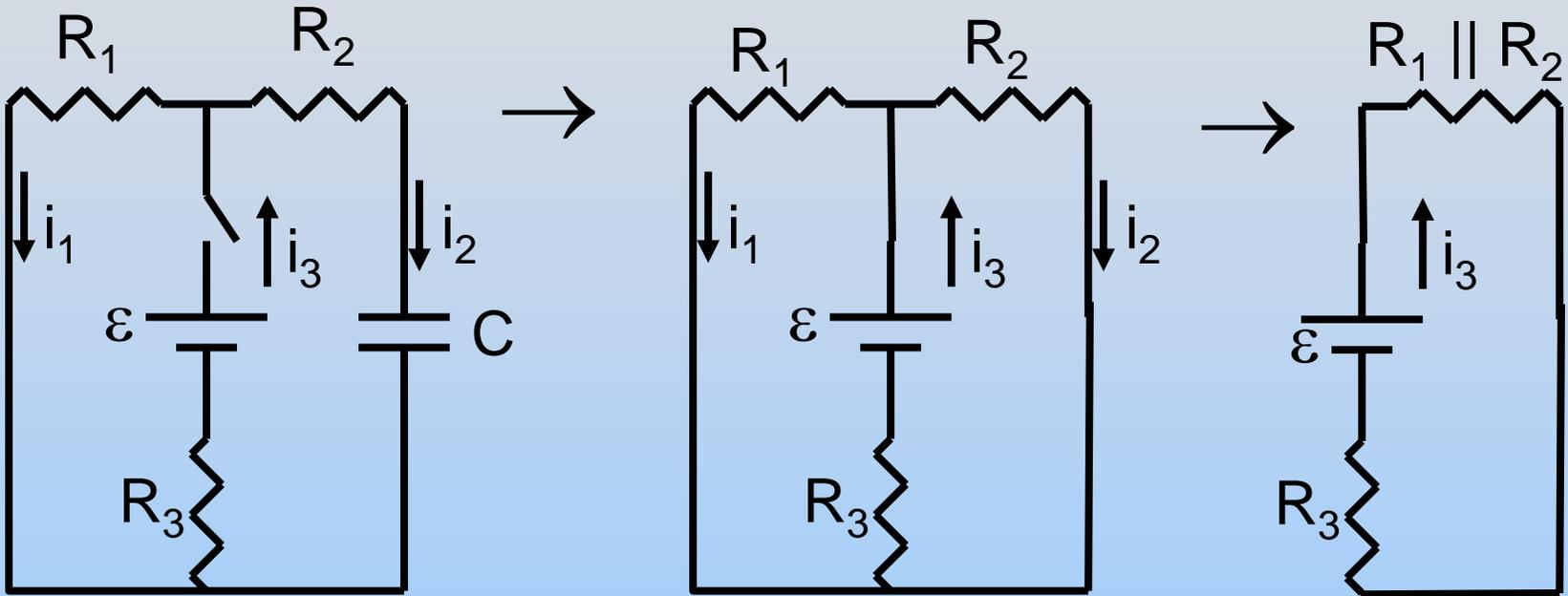
$$R_{\text{eq}} = R_3 + \frac{1}{\frac{1}{R_1} + \frac{1}{R_2}} \Rightarrow i_3 = \frac{\varepsilon}{R_{\text{eq}}}$$
