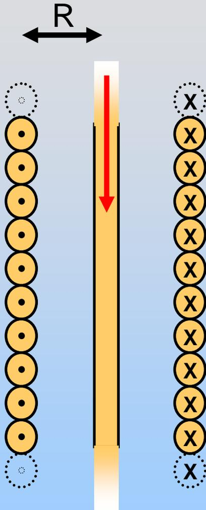
A current  $I$  flows up a very long solenoid and then back down a wire lying along its axis, as pictured. The wires are negligibly small (i.e. their radius is 0) and are wrapped at  $n$  turns per meter.
