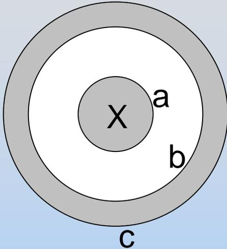
Consider a coaxial cable of with inner conductor of radius  $a$  and outer conductor of inner radius  $b$  and outer radius  $c$ . A current  $I$  flows into the page on the inner conductor and out of the page on the outer conductor.
