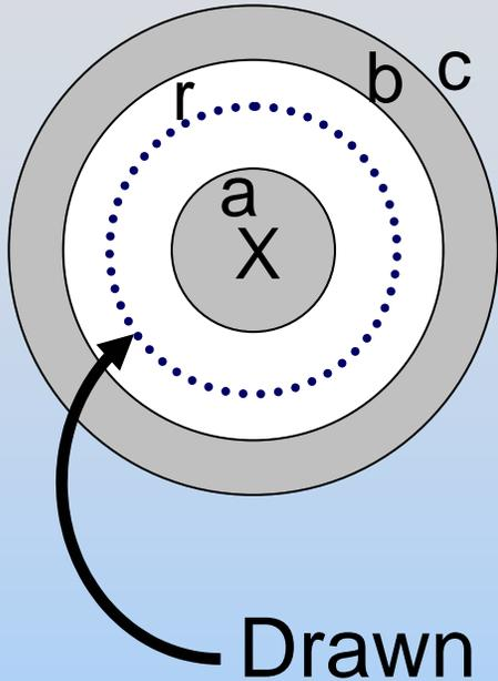
Everywhere the magnetic field is clockwise. To figure out the magnitude use Ampere's Law:
