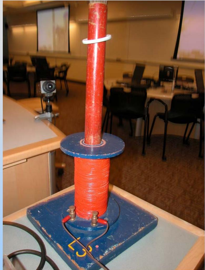
An aluminum ring jumps into the air when the solenoid beneath it is energized
