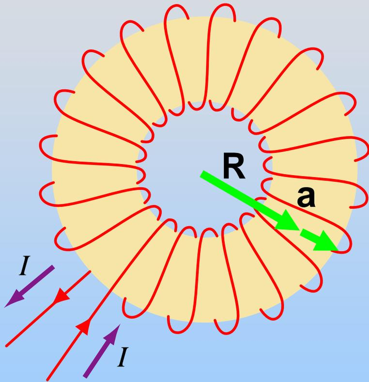
A torus (a solenoid of radius  $a$  and  $n$  turns/meter whose ends are bent around to make a donut of radius  $R$ ) carries a uniform current  $I$ .
