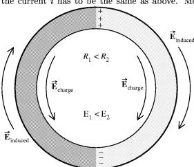
charge conservation. But the electric field in the left half of the wire loop  $(\vec{\mathbf{E}}_1)$  must now be **different** from that in  $\vec{\mathbf{E}}_{\text{induced}}$  the right half  $(\vec{\mathbf{E}}_2)$ .
