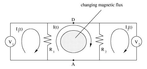
A magnetic field is present in the shaded area; it is perpendicular to the page, and it is changing in time. There are two identical voltmeters  $V_1$  and  $V_2$ , and two resistors  $R_1$  and  $R_2$ ; the internal resistance of each voltmeter,  $R_i$ , is much much larger than  $R_1$  and  $R_2$ . All connecting wires have a negligible resistance.
