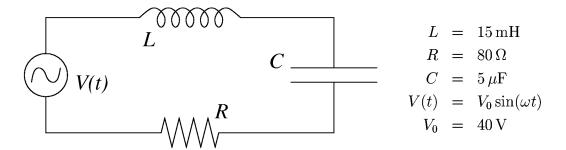
(a) As discussed in lecture (and in Giancoli Section 31-6, p. 780), in an *LRC* circuit, the driving frequency at which the current reaches a maximum (resonance) is
