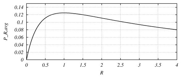
As stated in the problem, the maximum power is delivered to a load when the load "impedance" (R) is equal to the generator impedance (r). In the case under consideration we are *not* delivering maximum power to the load because  $R \gg r$ . Our given values for R, r, and  $\mathcal{E}_0$  yield
