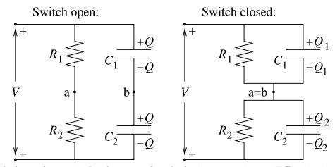
Define symbols as shown in the diagram, for algebraic convenience. Effective circuits for the open-switch and closed-switch cases are shown.
