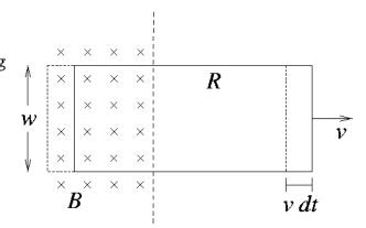
In a small time interval dt, the loop moves a distance v dt, and thus the area of the loop within the B-field region decreases by an amount dA = wv dt. The field magnitude remains constant, so the magnetic flux through the plane surface bounded by the loop decreases by an amount  $d\Phi_B = B dA = Bwv dt$ . By Faraday's law (Giancoli Equation (29-2a), p. 736), the magnitude of the induced emf will be
