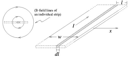
To solve for the magnetic field of a current-carrying ribbon, we break it up conceptually (and mathematically) into many infinitesimal strips which may be regarded as wires. The principle of linear superposition tells us that the magnetic field of the ribbon will be the vector sum of the magnetic field contributions of the individual strips.
