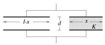
(a) To get the total capacitance of this arrangement, we consider it to be the equivalent of two capacitors in <u>parallel</u>, as shown above. The "capacitor" on the left (no dielectric) has plate area l(l-x) and (by Giancoli equation 24-2, p. 615) capacitance  $\epsilon_0 l(l-x)/d$ . The "capacitor" on the right (with dielectric) has area lx and capacitance  $K\epsilon_0 lx/d$ . Thus the total capacitance is the sum of these:
