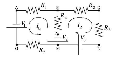
$$(R_1, R_2, R_3, R_4, R_5) = (10, 30, 50, 70, 100)\Omega$$
