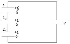
By the same sort of charge-conservation argument as in problem 3.1, all three capacitors must necessarily have the same charge  $\pm Q$  on their plates. Since all three have the same capacitance as well (call it "C"), we have
