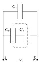
(a) First we find the equivalent capacitance  $C_{23}$  of the  $C_2$ - $C_3$  combination. These two capacitors are combined in series, so we have
