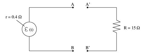
(a) If the load resistor  $R=15\,\Omega$  (with A connected to A', and B to B'), what average power will be delivered to the load?
