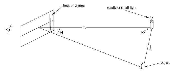
(g) Observe the two first order spectra as before (grooves in grating vertical). Now rotate the grating about the vertical; you observe an increase in  $\theta$ . Why?
