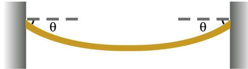
The curve of the clothesline, or of any flexible cable hanging under its own weight, is called a *catenary*.
