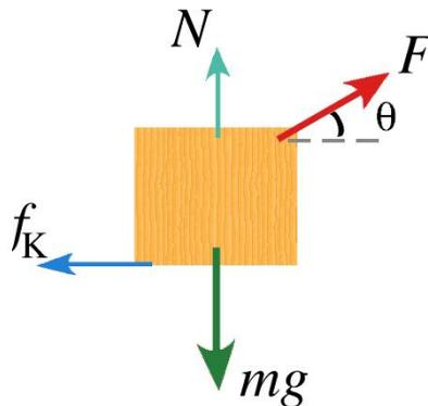
There's no acceleration in the vertical direction, so the sum of the vertical forces must be zero, i.e.  $N - mg + F \sin \theta = 0$ . This gives us  $N$ , which we don't know the value of, in terms of  $F$ , which we also don't know the value of (yet).
