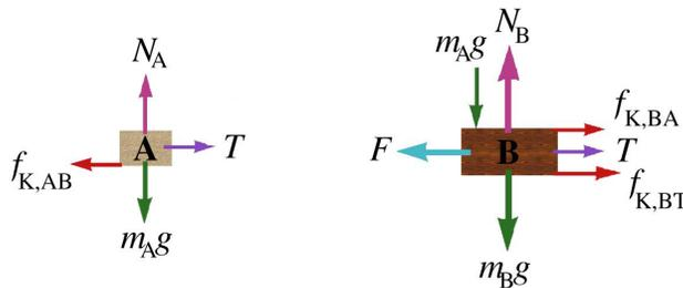
If block B is to move with no acceleration, then due to the cord block A must undergo no acceleration. Thus the total force on each block will be zero. Let's write down the equation for the horizontal motion of block B and see what we need to figure out.
