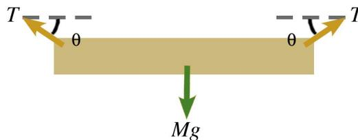
A symmetry argument can be used to demonstrate that both short ropes must be under the same tension  $T$ . That is to say the physical situation is identical if one looks instead at the left-right mirror image of the problem, so there's no way the two ends' tensions can be unequal.
