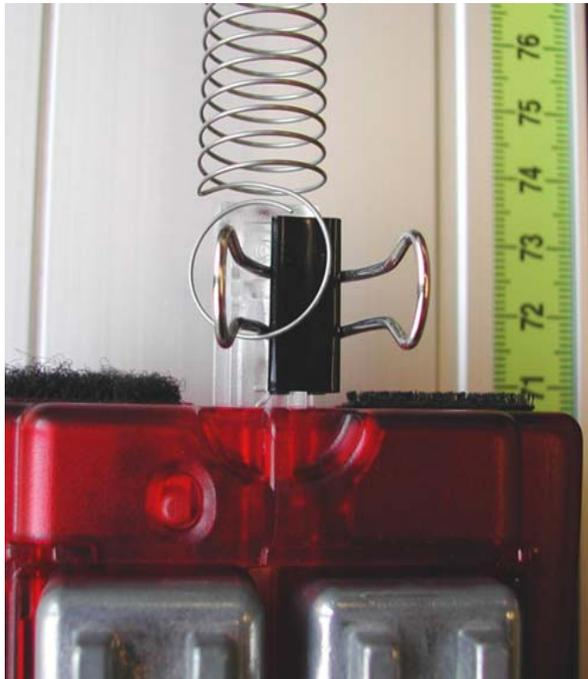
Attach spring to plunger on cart with a binder clip and to the hook on force sensor.
