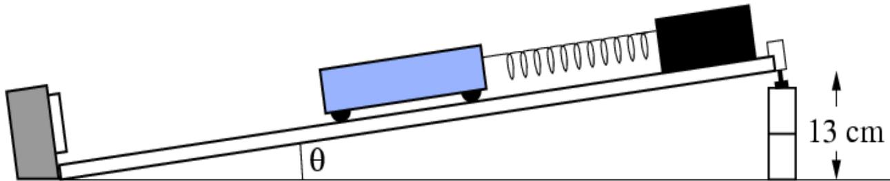
Unclip motion sensor, raise the force sensor end of track
