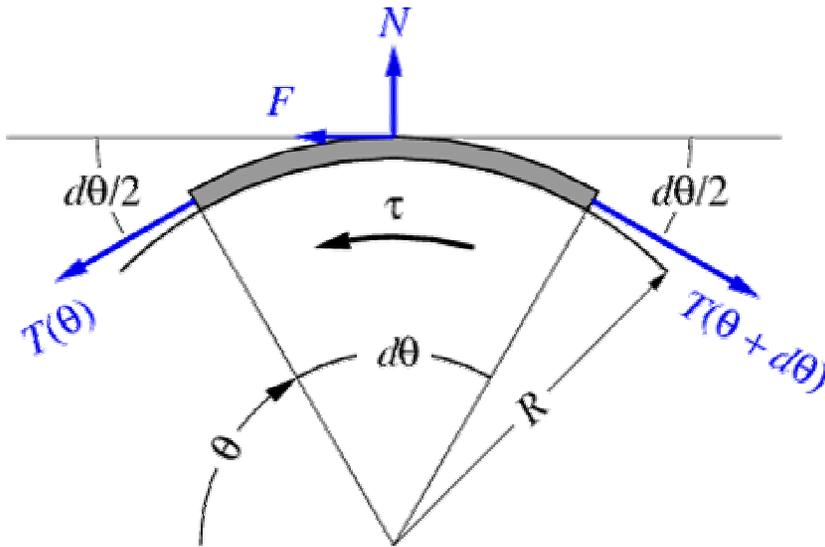
To investigate the friction of a string wrapped around a cylinder, observe that it increases exponentially, and to measure the friction coefficient  $\mu$ .
