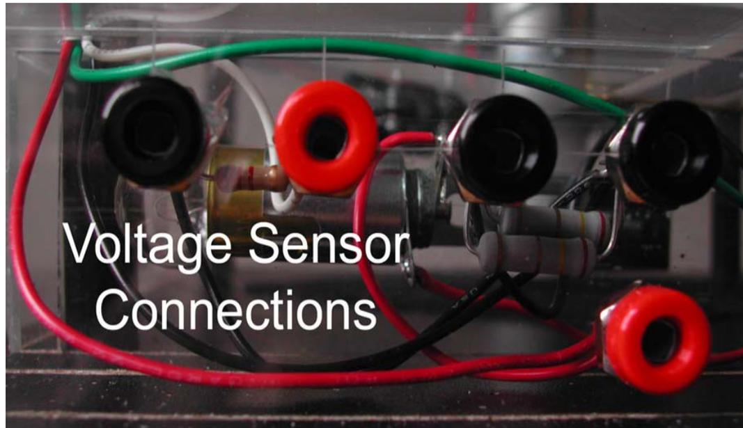
Connect the voltage sensor to the left side banana jacks!
