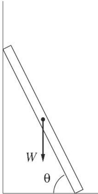
A uniform ladder (one whose center of mass is at its geometrical center) of weight  $W$  leans against a wall at an angle  $\theta \approx 60^\circ$  up from the ground. The coefficient of friction between the ladder and the ground is  $\mu_G$  and between the ladder and the wall is  $\mu_W$ . The magnitudes of these two coefficients are about equal.
