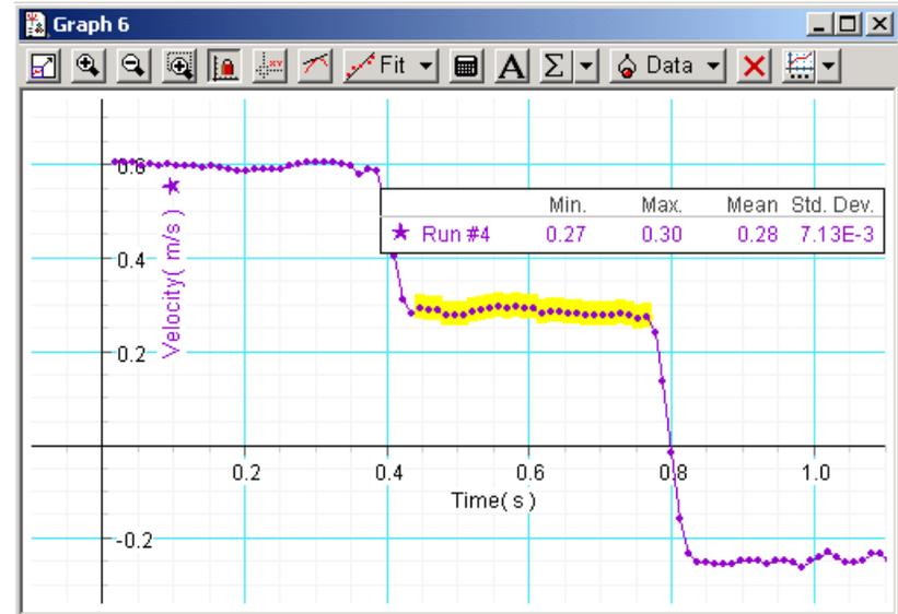
Use Statistics Tool ( $\Sigma$ ) to measure velocities  $v_{A,1}$  and  $v_2$ , before and after the collisions. Complete the table.
