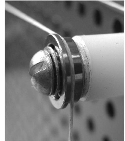
Increase ccw torque on cylinder smoothly to the slipping point, then turn slowly for 1 or 2 seconds.
