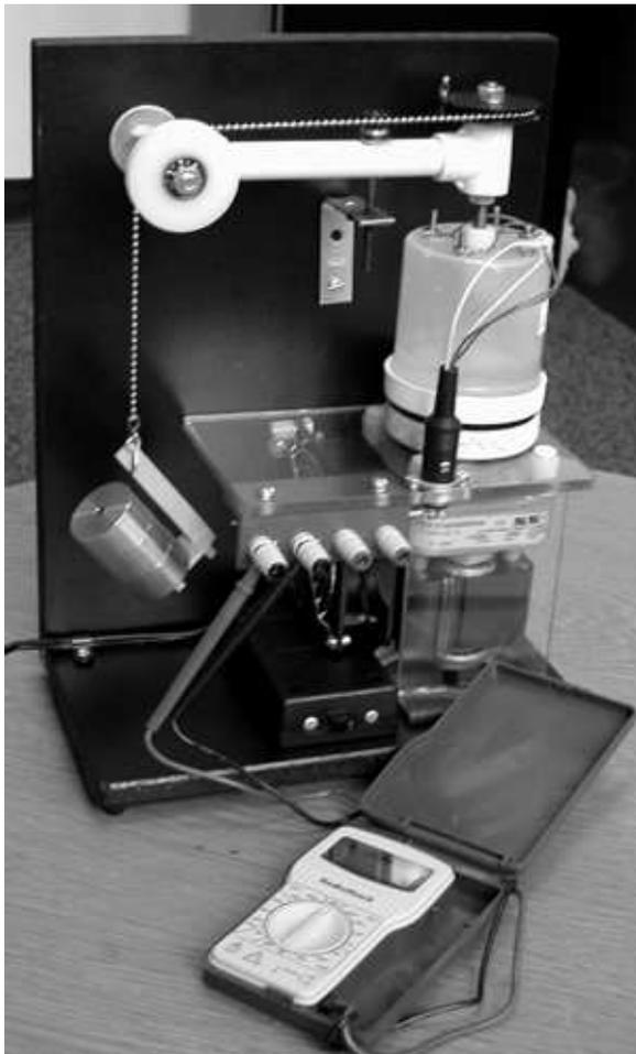
The photo shows the apparatus. A motor rotates a plastic pot scrubber against a thin metal disk that forms the bottom of the plastic reservoir that contains the water, and the work done by the friction warms the water. A thermistor immersed in the water enables you to measure its temperature.
