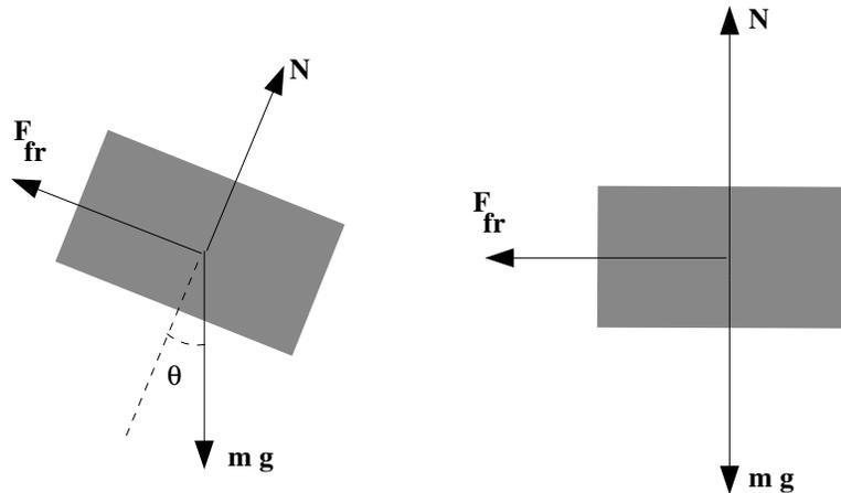
Figure 1: Free-body diagrams for the block sliding on the inclined plane (left) and the same block on the horizontal plane (right)
