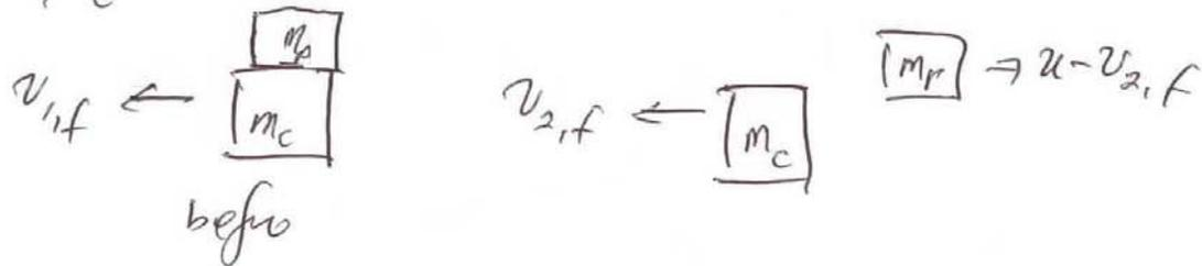
$$\hat{c}: 0 = p_2 - p_1 = (m_p (u - v_{2,f}) - m_c v_{2,f}) - (-(m_c + m_p) v_{1,f})$$
