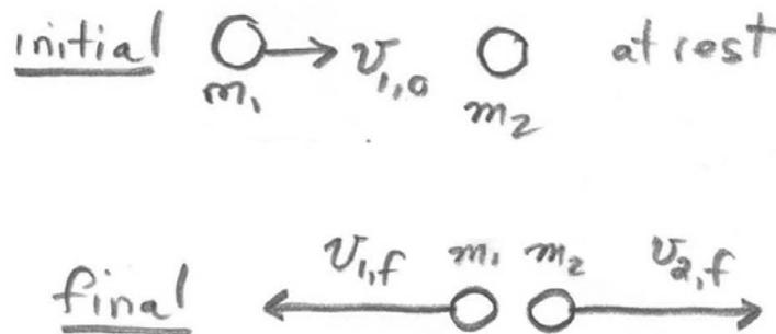
**Figure 10.11** Momentum flow for a one-dimensional collision.
