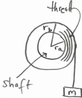
a) Suppose a mass  $m = 5.0 \times 10^{-2} \text{ kg}$  stalls the motor when the wound thread has an outer radius of  $r_f = 2.4 \times 10^{-3} \text{ m}$ . Calculate the stall torque.
