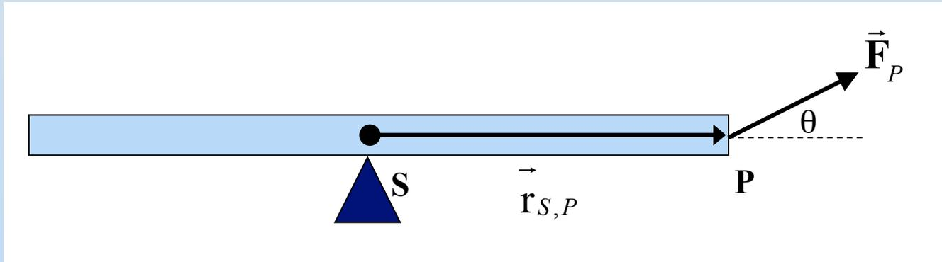
Torque about point  $S$  due to the force exerted at point  $P$ :
