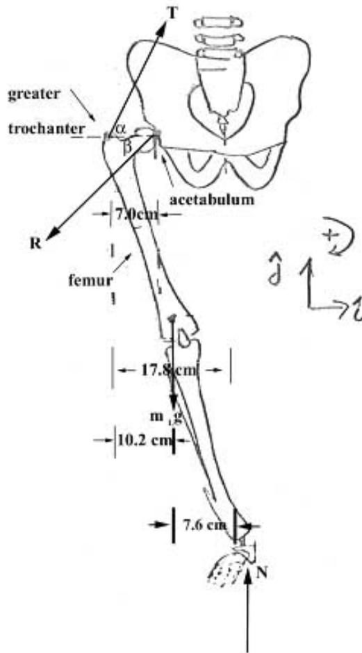
The direction  $\alpha$  is given. After drawing your free body diagram for the right leg, you are trying to decide what point to compute the torques about. Explain the disadvantages /advantages if you chose each of the points listed below.
