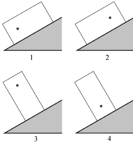
**Answer 3.** In order to tip over, the box must pivot about its bottom left corner. Only in case 3 does the torque about this pivot (due to gravity) rotate the box in such a way that it tips over.
