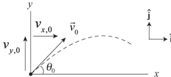
**Figure 6.16** A vector decomposition of the initial velocity
