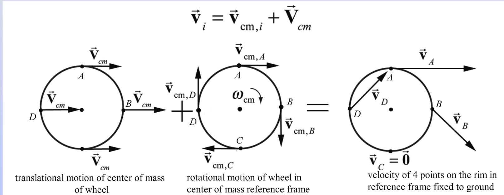
The velocity of the point on the rim that is in contact with the ground is zero in the reference frame fixed to the ground.
