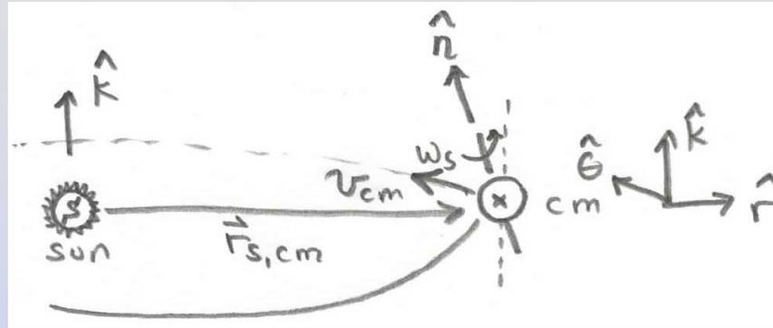
For a body undergoing orbital motion like the earth orbiting the sun, the two terms can be thought of as an orbital angular momentum about the center-of-mass of the earth-sun system, denoted by S,
