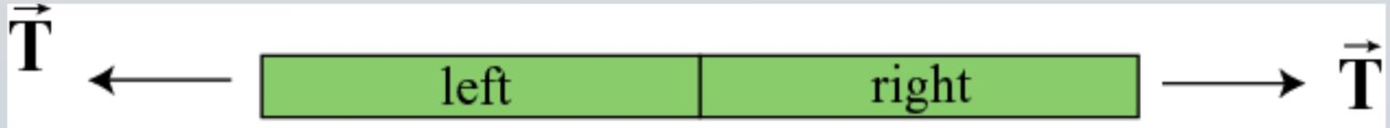
The *tension* in a rope at a distance  $x$  from one end of the rope is the magnitude of the action-reaction pair of forces acting at that point ,
