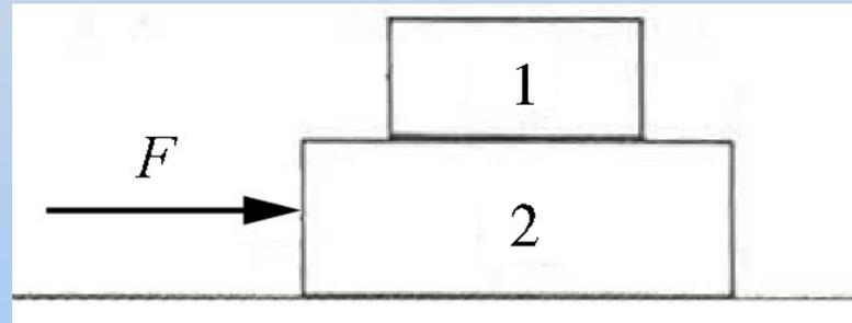
A horizontal force of magnitude  $F$  is applied to the lower book so that the two books move together without slipping. Identify all action-reaction pairs of forces in this problem and draw free-body force diagrams on each object.
