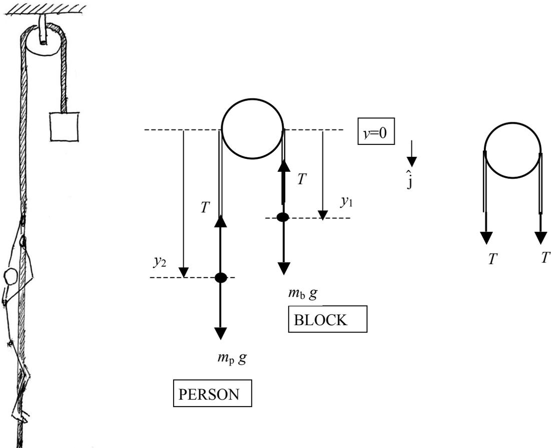
The force diagrams are shown in the above figure. As the person pulls up on the rope, there is a force down on the rope, creating a tension in the rope. This tension is transmitted through the rope, and so is also the force on the object. Both the person and block satisfy Newton's Second Law,
